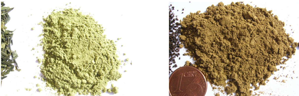
Fig. 4: After three minutes the results shown in the photos were achieved. Immediately after opening the grinding bowls the temperature was taken and the values were just below 40 ° C.
