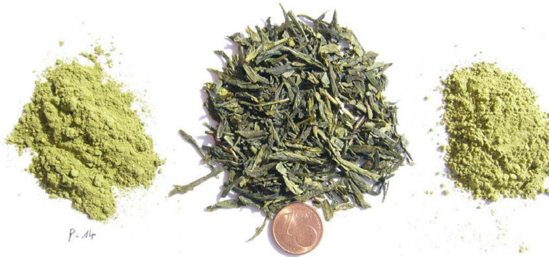
Fig. 5: On the left is the comminuted sample processed with the Variable Speed Rotor Mill PULVERISETTE 14 and on the right the sample comminuted with the Planetary Micro Mill PULVERISETTE premium line.
