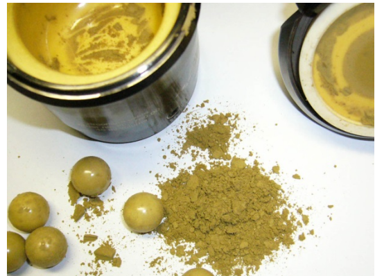
Fig. 3: Grinding bowl and grinding balls made of zirconium oxide
