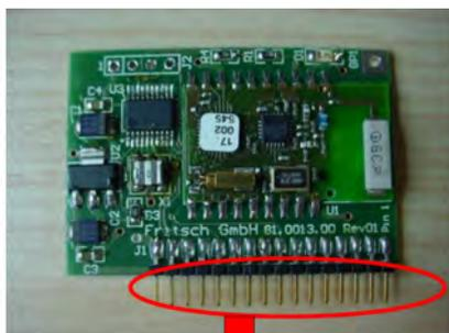
3. ➤ Insert the receiver module in the corresponding slot. (As illustrated)
