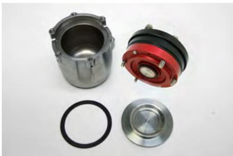
4. ➤ If the lid (9) is on the unit, release it by hand and place it to the side. The lid normally remains on the bowl (10).
