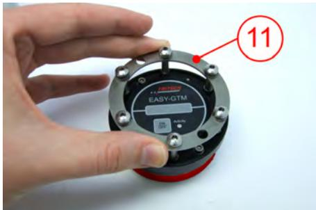
Remove the locking ring including the screws of the measuring/transmission unit and clean it completely.
