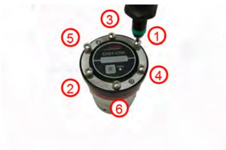
4. ➤ Tighten the socket-head screws crosswise with a torque spanner (1) until it disengages! To be on the safe side, re-tighten all screws again after initially tightening them. All screws are secured against becoming loose during the grinding process once they have been tightened with the torque spanner as described.
