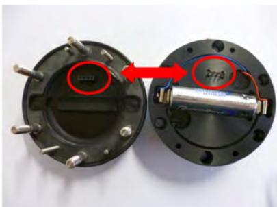
8. Close the battery compartment! Make sure the plug contacts are in the correct position!
