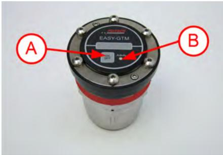
1. ➤ If not already done, switch off the radio system using the button (A). The LED (B) goes out.
