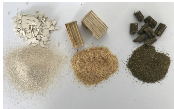
Fig. 4: Samples of plastic, wood- and feed pellets: Comminuted with the rotor with notched edges and a sieve cassette with 0.75 mm trapezoidal perforation
