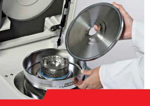
Fig. 1: Inside of PULVERISETTE 14 rotor mill, showing fixed collection pan, rotor, and sieve ring. High performance Cyclone sample collector in stainless steel is shown on the left. Used together with modified collection pan, the P14 system and Cyclone allow continuous feeding and homogenization of flowers or CBD isolate into the low micron range (consistency of talcum powder).
