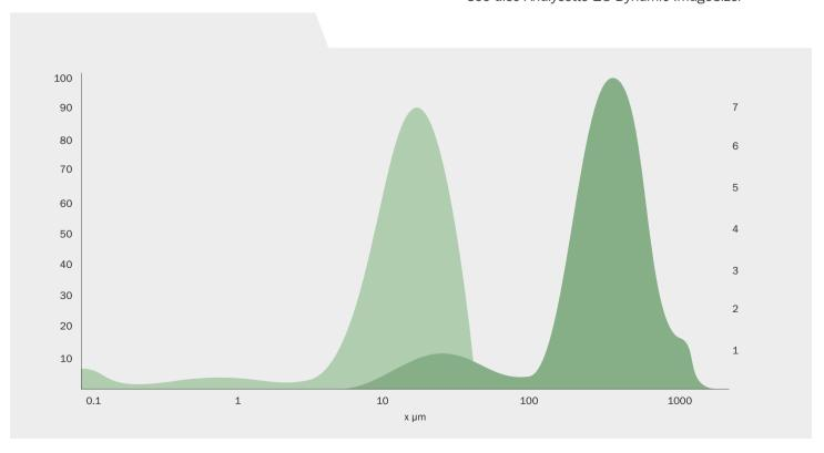
Fig. 2: The ANALYSETTE 22 NanoTec was used to measure CBD isolate before and after homogenization. Starting CBD sample (dark green) contained a mixture of loose granules with a wide particle size distribution. Material homogenized using the PULVERISETTE 14 classic line variable speed rotor mill (light green) resulted in a particle size consistency similar to talcum powder.
