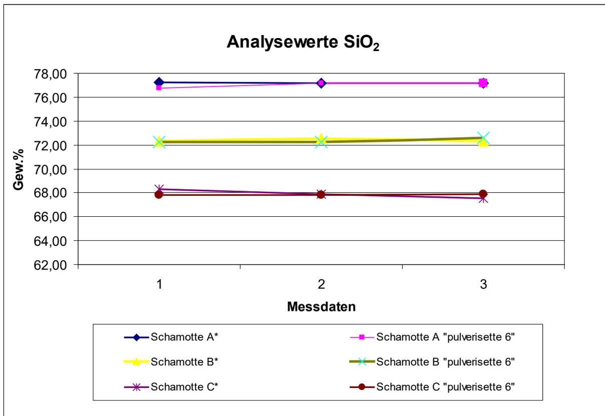
Illustration A: Comparison of the **weight** % of SiO<sub>2</sub> of various fireclays from past preparation methods (firing clays A\*-C\*) prepared with the FRITSCH Planetary Mono Mill PULVERISETTE 6 classic line.
