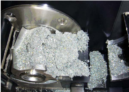
Fig. 1: After the preparation only a little material may remain in the grinding chamber of the Cutting Mill. On no account may it look like
