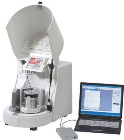
Planetary Mono Mill PULVERISETTE 6 *classic line*
