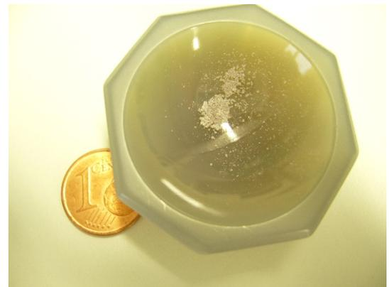
Fig. 2: A fine powder was obtained after 3 minutes of comminution
